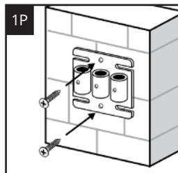
**Secure Mounting Plates To The Wall**
