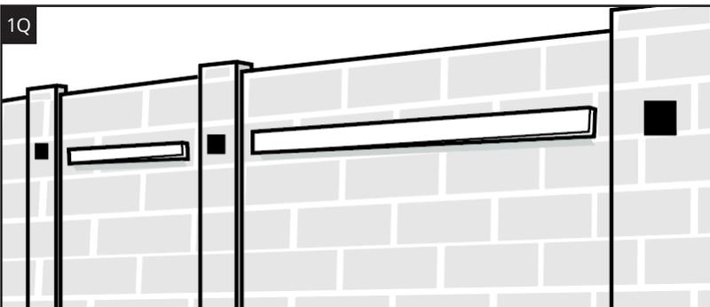
**Note:** *If possible, align the holes of the mounting plate along a mortar joint. This will make repair easier if the Purrfect Fence is removed.*
