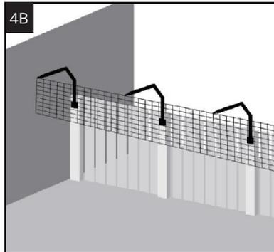
**Install Mesh Fence One Side at a Time**
